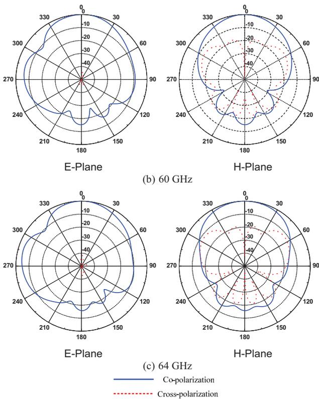
Fig. 5: Simulated antenna radiation pattern at 57 GHz, 60 GHz and 64 GHz.
