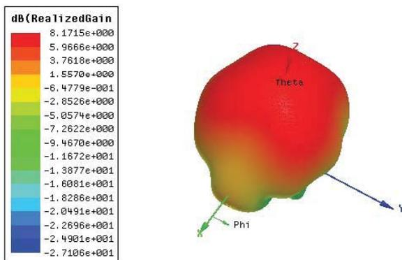
Fig. 6: 3-D radiation pattern at 60 GHz.
