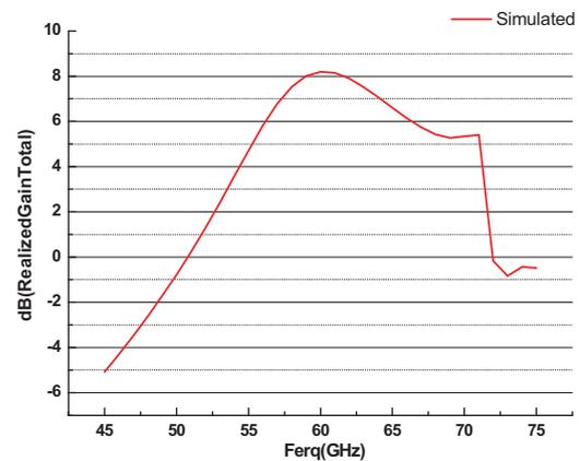
Fig. 4: Simulated realized gain total of the antenna.
