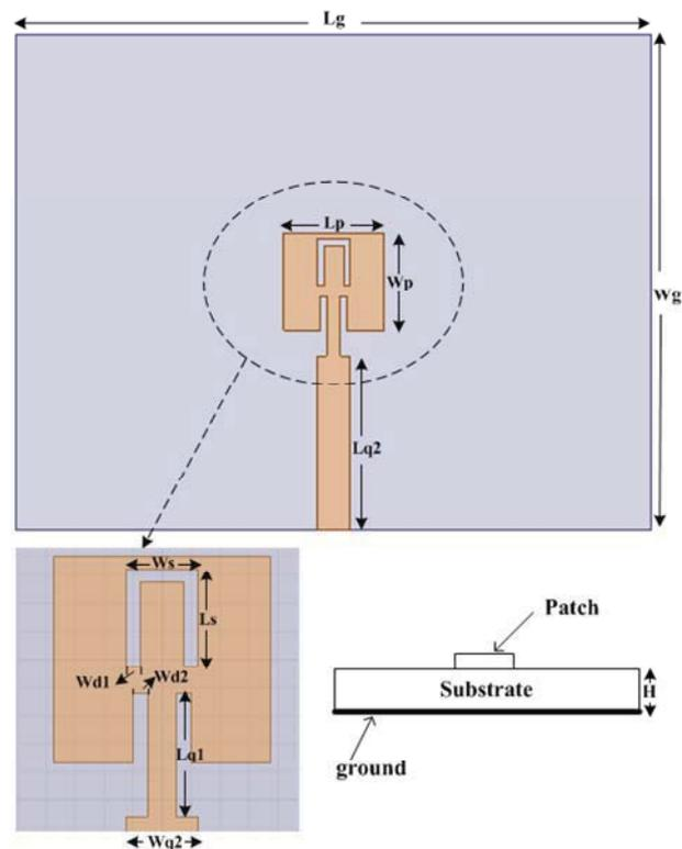
Fig. 1: The structure of the antenna.
